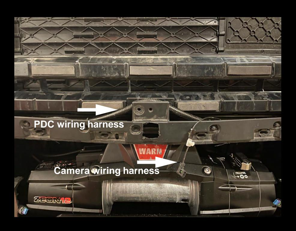
Put the PDC wiring harness back in place, run the camera wiring hares through the new hole, bolt the bumper cover center bolt back down, connect the camera to the wiring harness and install the grill.
