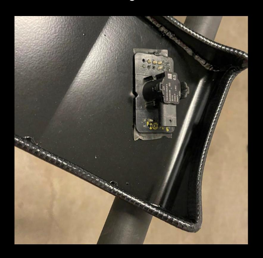
Find the PDC wiring on each side of the bumper and free up as much slack as available and set to each side of the winch tray.
