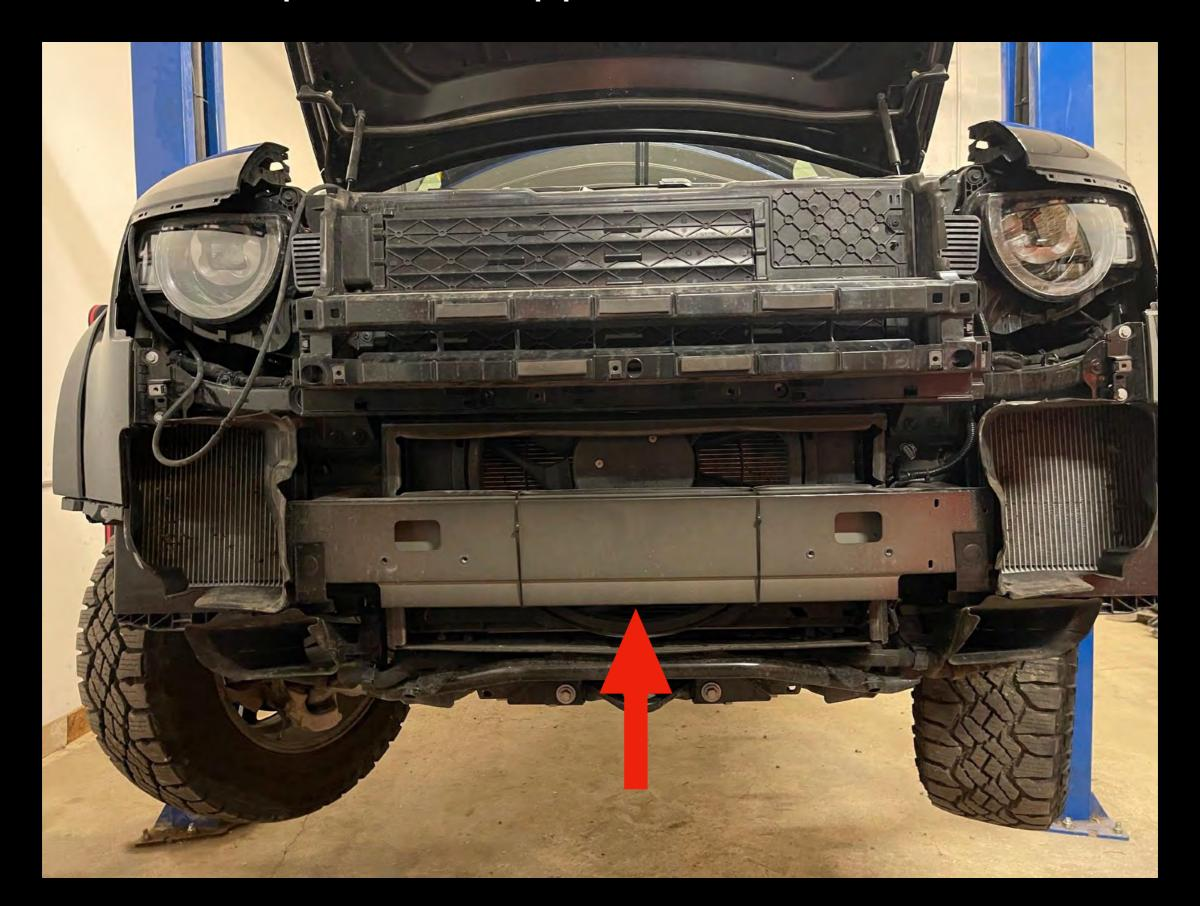
Remove the two clips on each side of the brake cooling duct.
