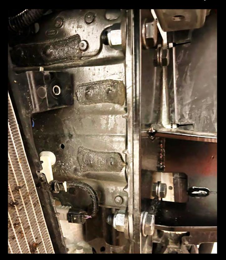
On the inside of the frame, access the top bolt from the engine bay and the lower from under the Defender. Reinstall the auxiliary radiators. When all eight bolts are in place torque to **100 Nm**
