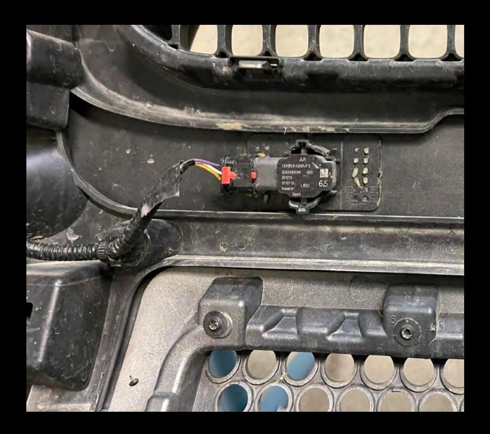
Gently pry up on the park sensor mounting bracket. The bracket is glued or taped (2-sided) in place.
