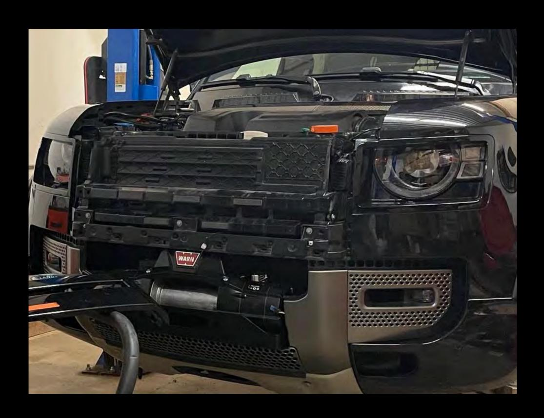
A hole needs to be drilled in the grill for the front camera you set aside earlier.
