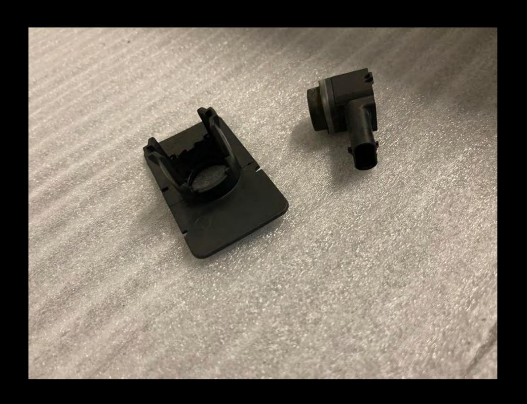
Using two sided tape mount the PDC to the vanity plate.
