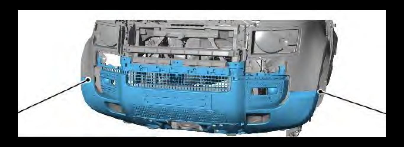
In the wheel wells, remove the fender liner.
