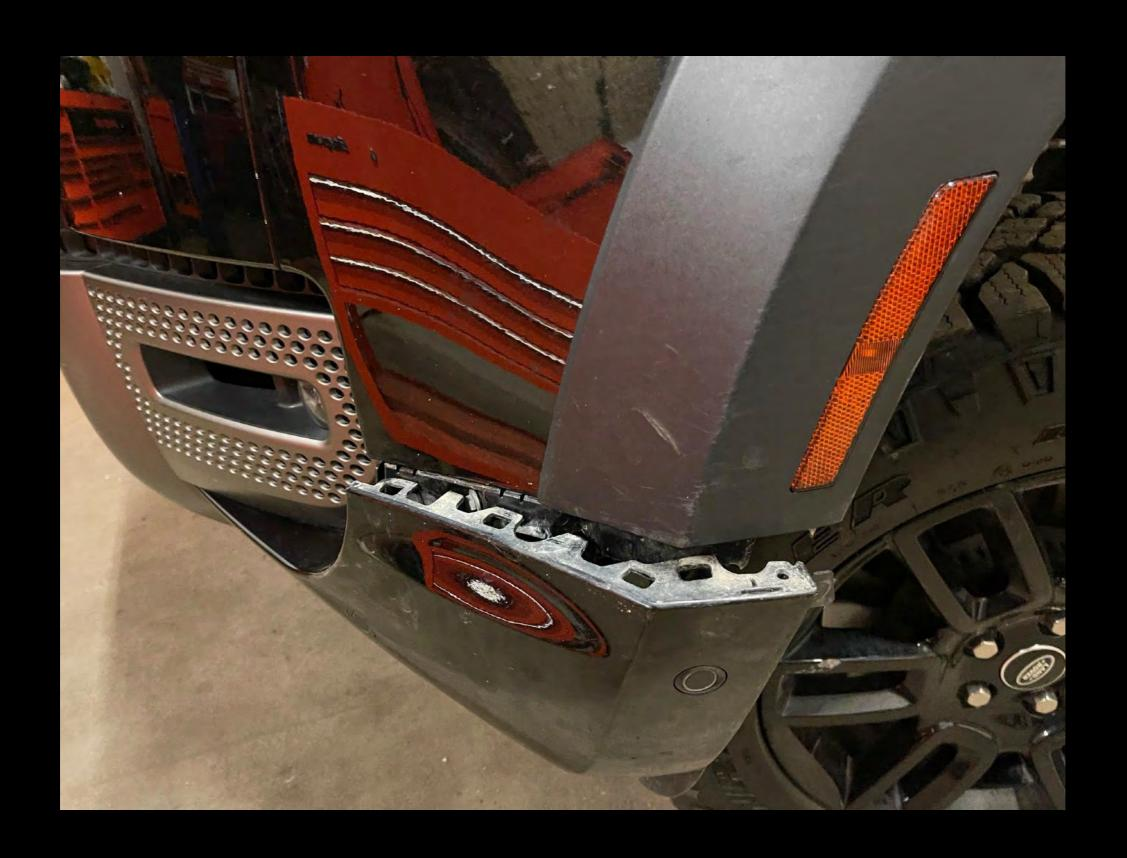
With the corners loose and center bolt removed pull the bumper cover off with some help from a friend.
