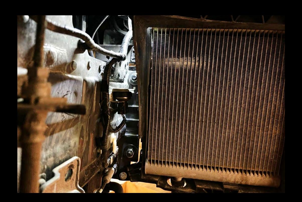
Reinstall the brake cooling ducts. Hold them in place with zip ties until the bumper cover is installed.
