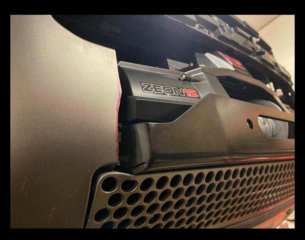
With everything trimmed, properly reinstall the two electrical connections on the left side of the bumper cover, the axillary radiators, bumper cover, wheel well liners, splash guards, and overflow bottle.
