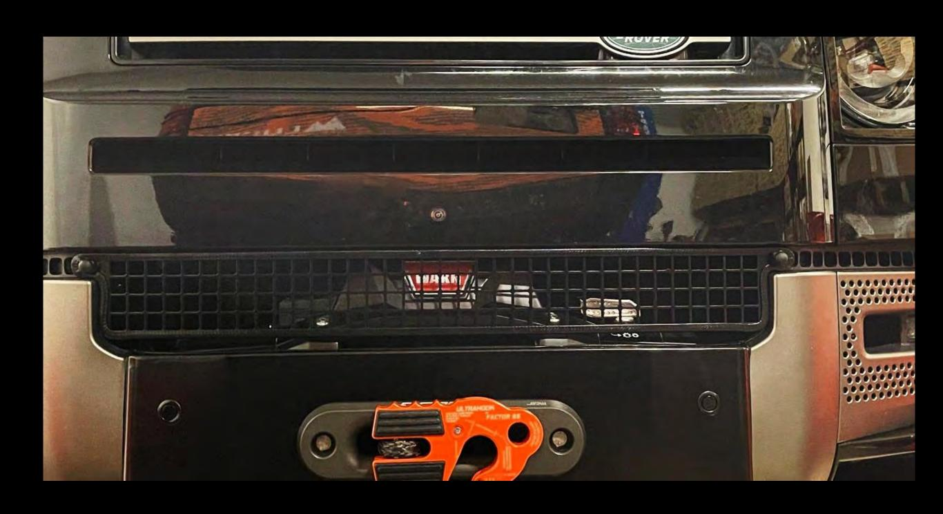
Clear the plastic out of the way behind the first square on each side so the bolt and washer will sit flush.
