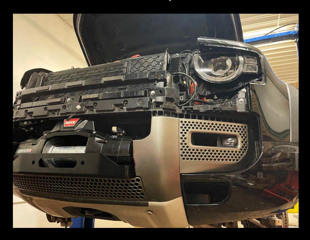
You may need to trim the bumper cover in this area so it does not hit the winch tray. Only remove what is needed. (See the next page before trimming.)
