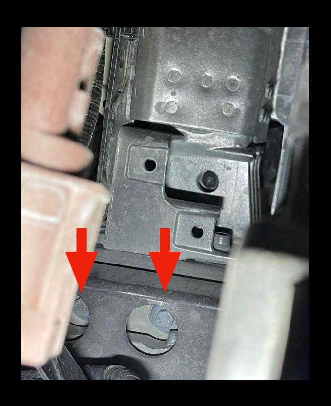
Remove the eight bolts holding the core support to the frame.
