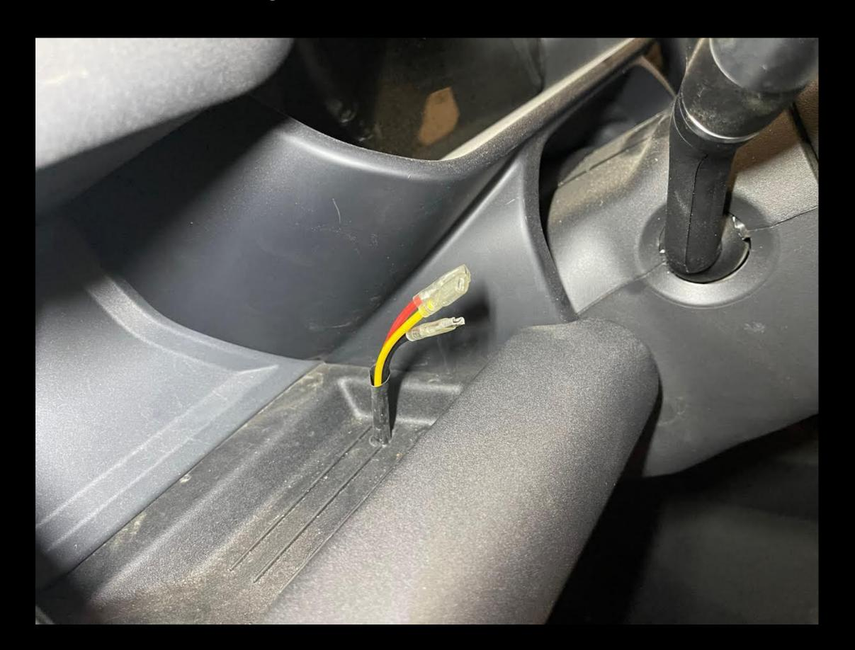
Connect the wires to the switch, clean off the instrument cluster bezel, remove the backing for the double-sided tape, and stick the pod to the bezel.
