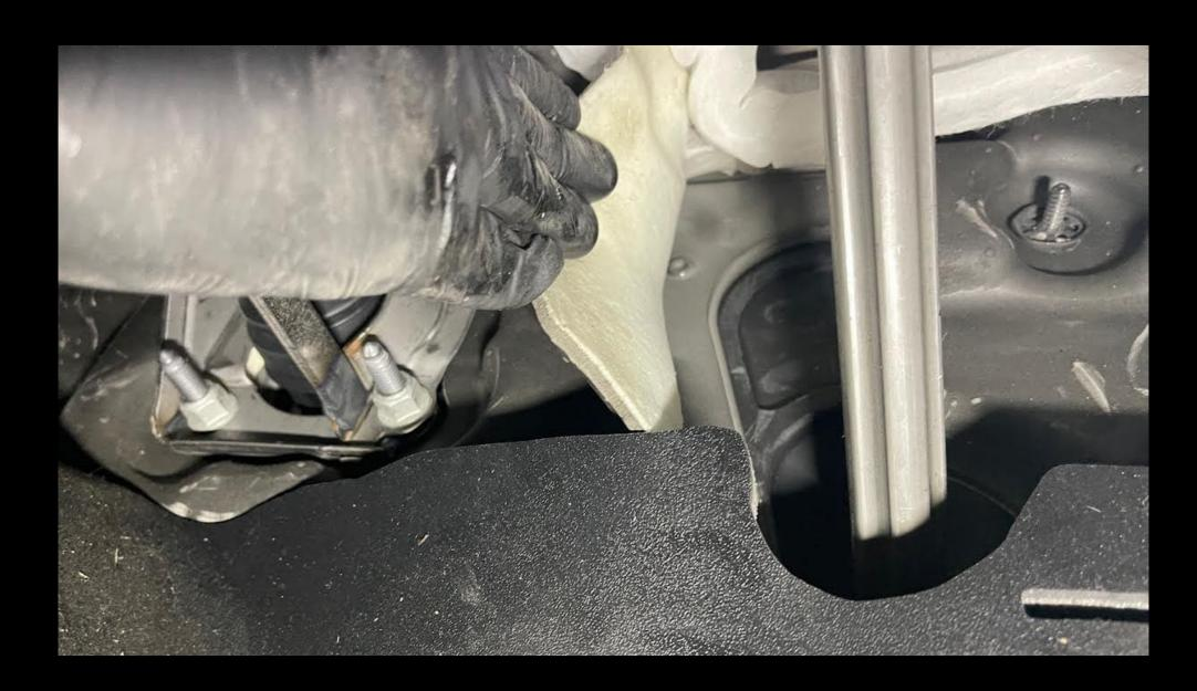
Gently poke a small hole in the rubber steering shaft boot under the letter "A" in then Land Rover Logo.
