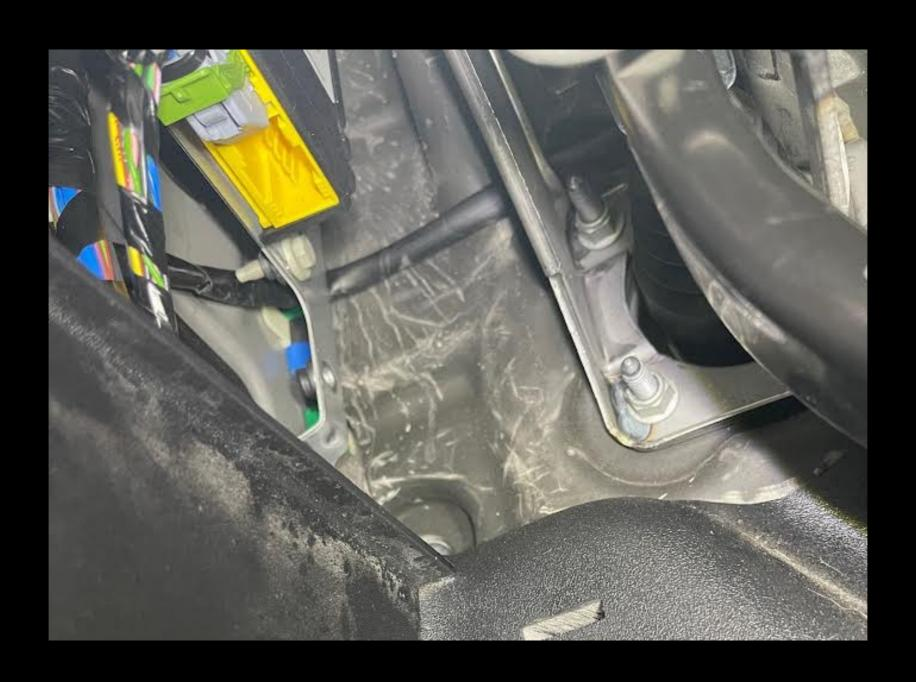
Gently pull back the dash trim piece. The trim is held in by two clips and a bolt. You cannot access the bolt with out removing the outer portion of the dash.
