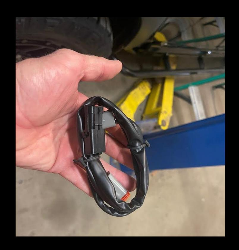
Connect the two harness to the four lights leaving the feed wire connector exposed on each side as shown.
