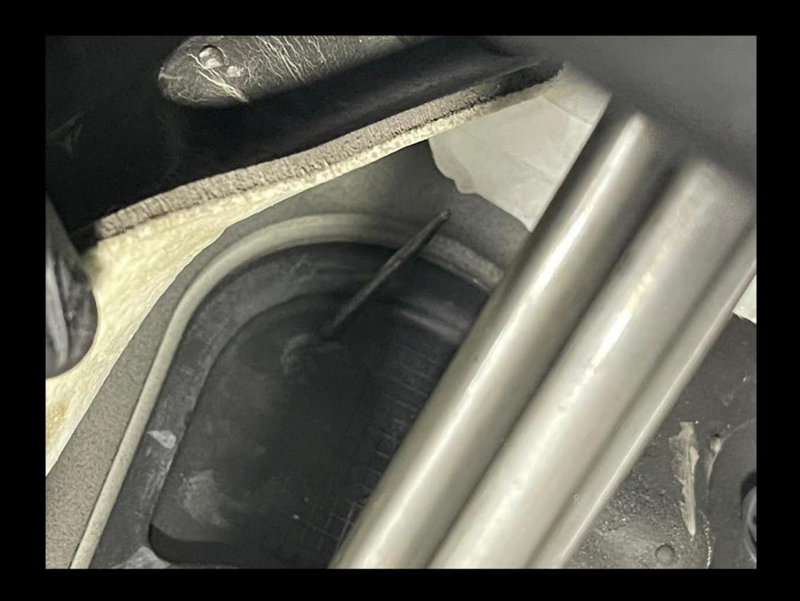
Enlarge the hole to accommodate the wiring harness, we recommend using a smaller wire to help fish the switch harness through the hole.
