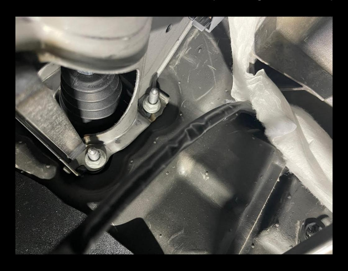
Run the wiring harness out of the way of any moving parts and sharp metal.
