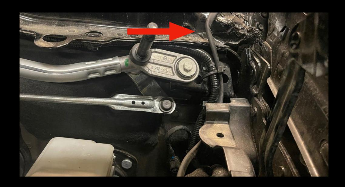
Attach the fused power feed to the auxiliary power port location "Red Arrow" and the ground to the top of the strut as shown "Blue Arrow".
