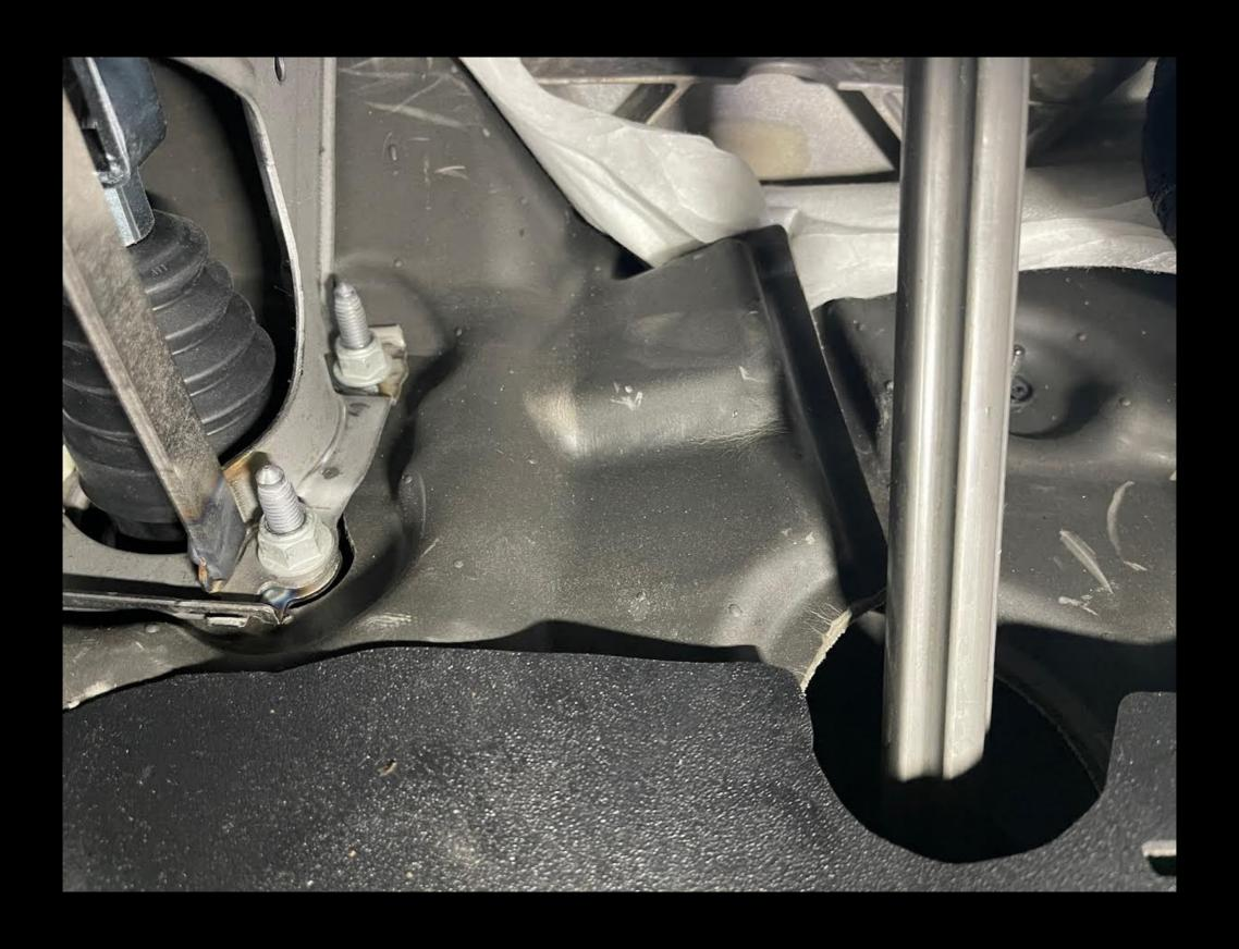
Pull back the padding to expose the steering shaft rubber boot.
