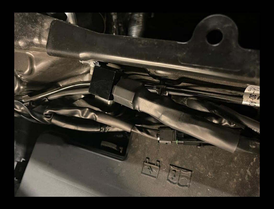
Remove the wires from the switch, note the location, so they can be re-installed in the same orientation.
