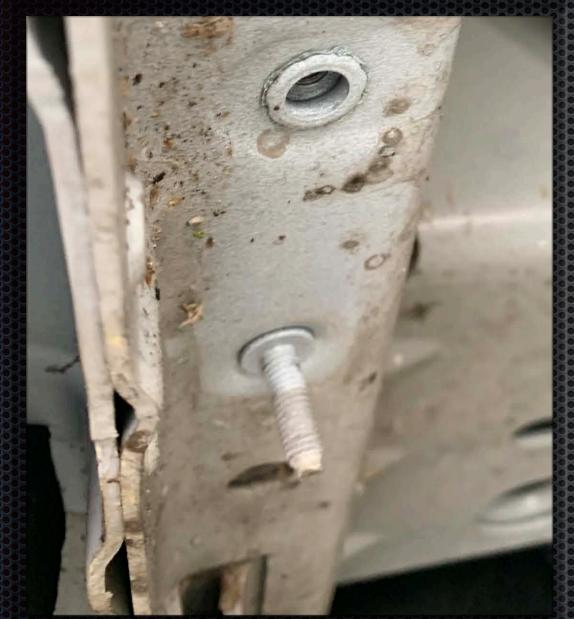
Snap off debris guards studs. We recommend vice grips. Debris guards can be reinstalled using new bolts in unused mounting points next to studs if desired.
