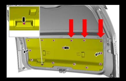
Locate and release the three top left tailgate trim panel retaining clips. (Red Arrows)
