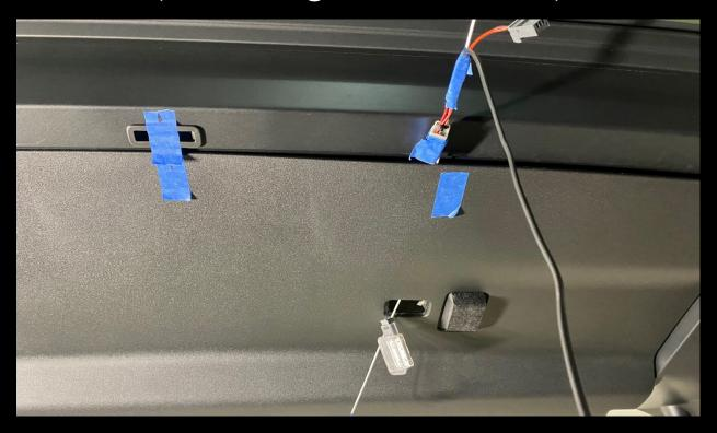
Tape bespoke OEM cable plug and socket adapter to the wire fishing tool
