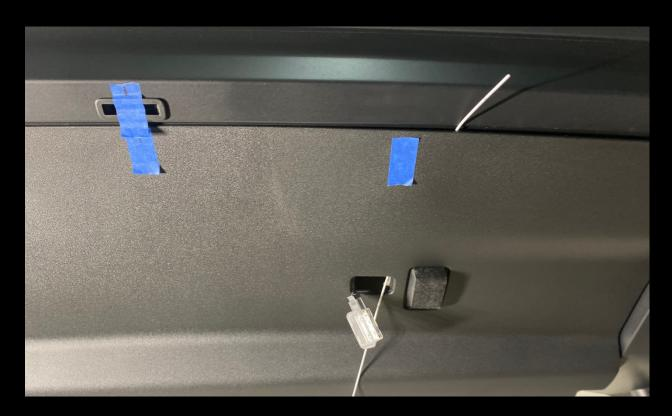
Insert a wire fishing tool behind the tailgate panel. (wire hanger shown here)
