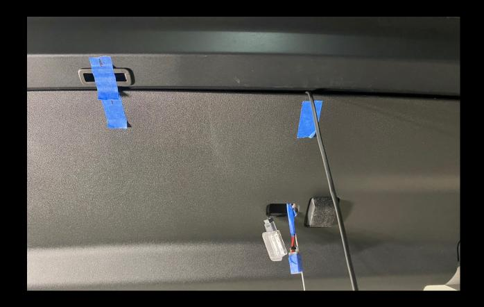
Gently pull the cable and socket adapter out the OEM LED light hole
