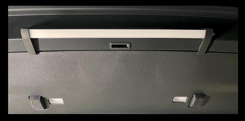
Firmly pop the top three tailgate retaining clips back into place.
