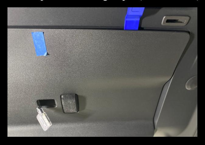
Use a plastic trim removal tool to get behind the panel to release the three retaining clips
