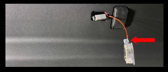
Plug the bespoke plug into the OEM LED light. (Red Arrow)
