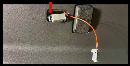
Plug the OEM cable into the bespoke socket adapter. (Red Arrow)
