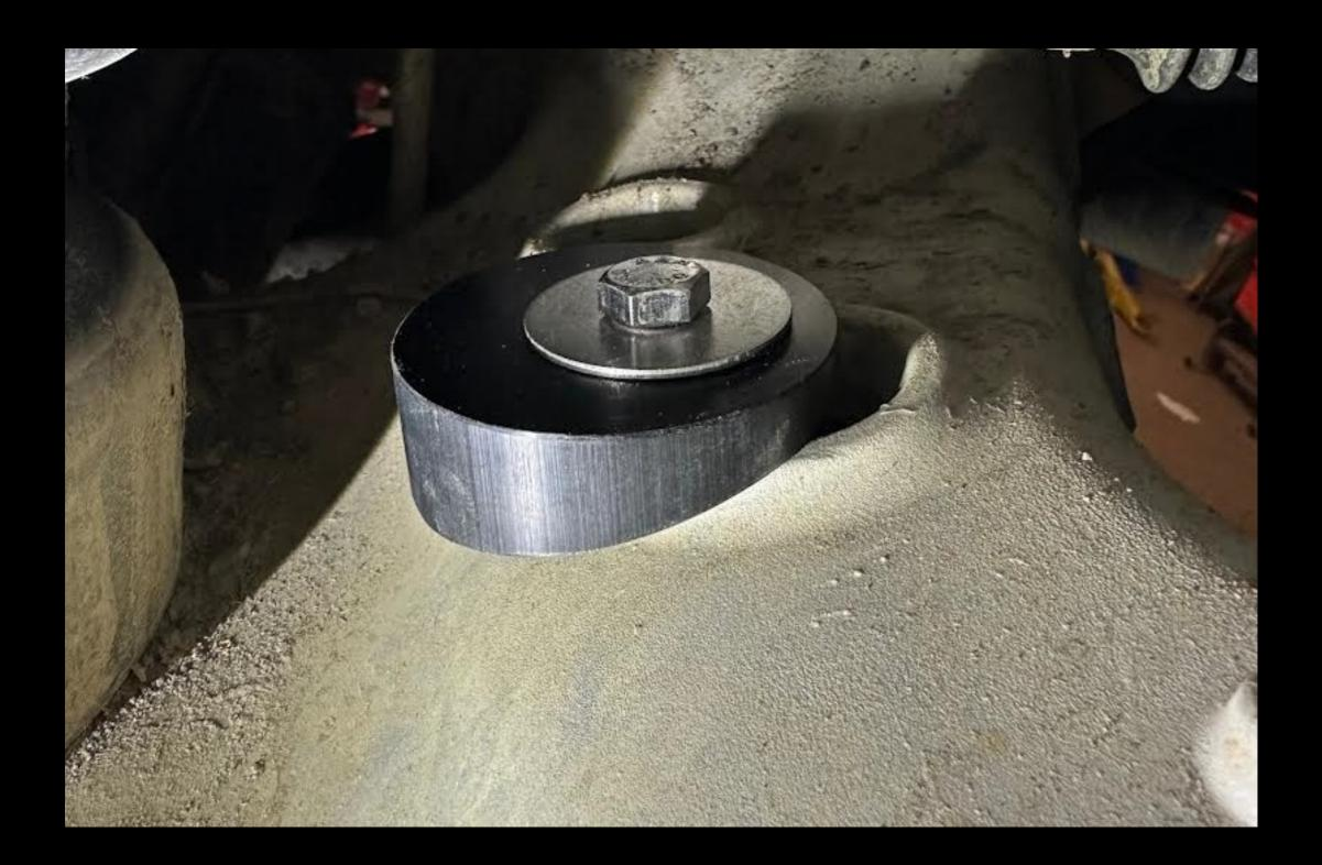
Align the bolt to the threaded nut. You can look through the hole in the control arm to make it easier.
