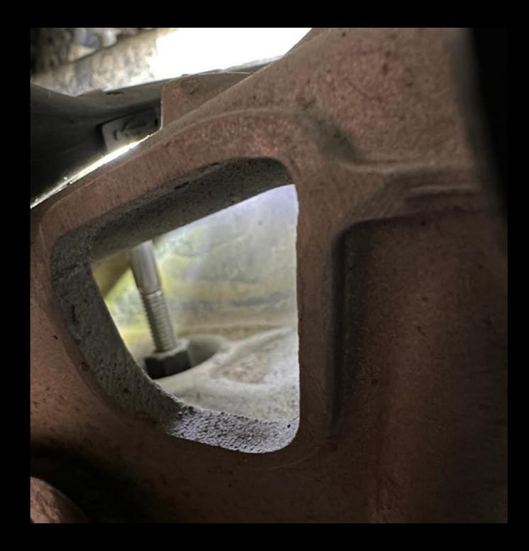
Tighten down the bolt, making sure the offset spacer keeps the bolt head flat on the washer. The casting bumps of the control arm will determine the rotation of the spacer. It does not need to be directly over the hole.
