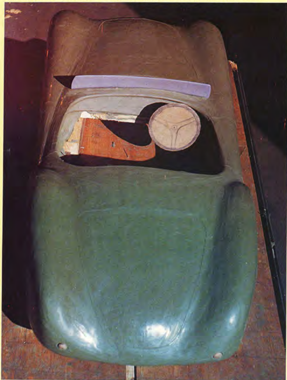
Rare contemporary photograph of an early 'C' type wind-tunnel model employed by Malcom Sayer; it shows an interesting stage in its development the cockpit is more like an XK 120's and there appears to be provision for an opening 'boot', plus a lift-out panel for engine access.
