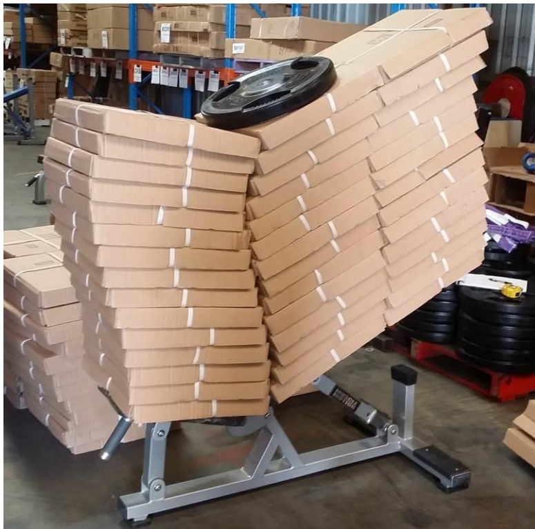
Figure: 3 Subject: View of the bench in the 30° incline position with the distributed test load (90140kg) applied.
