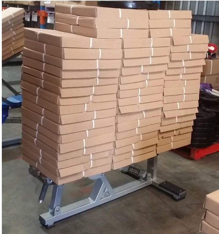
Figure: 2 Subject: View of the bench in the flat position with the distributed test load (1125.80kg) applied.
