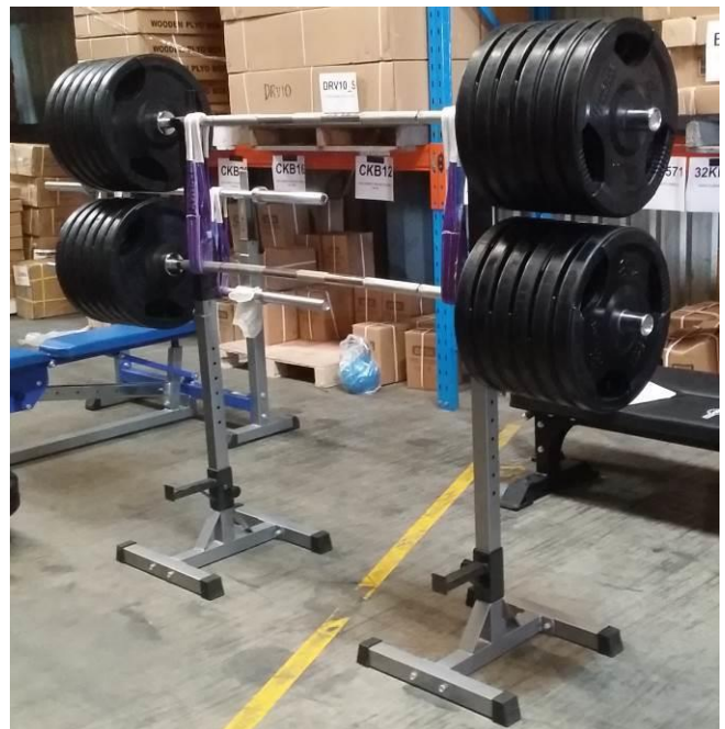
Figure: 2 Subject: View of the adjustable barbell stands with the distributed test load applied.
