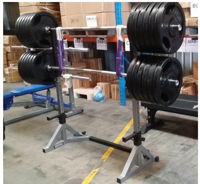
Figure: 2 Subject: View of the adjustable barbell stands with the distributed test load applied.
