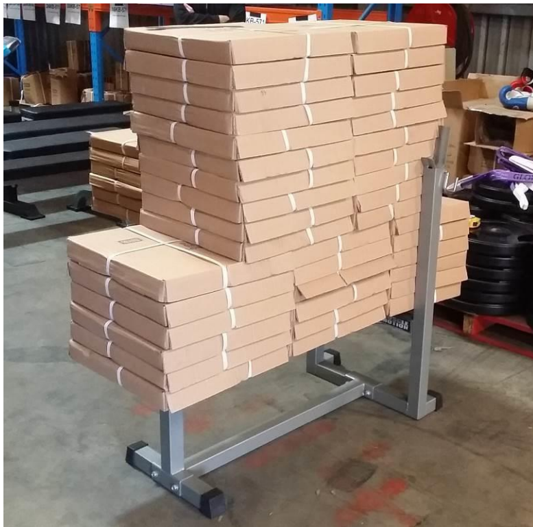
Figure: 2 Subject: View of the bench with the distributed test load (775.20kg) applied.
