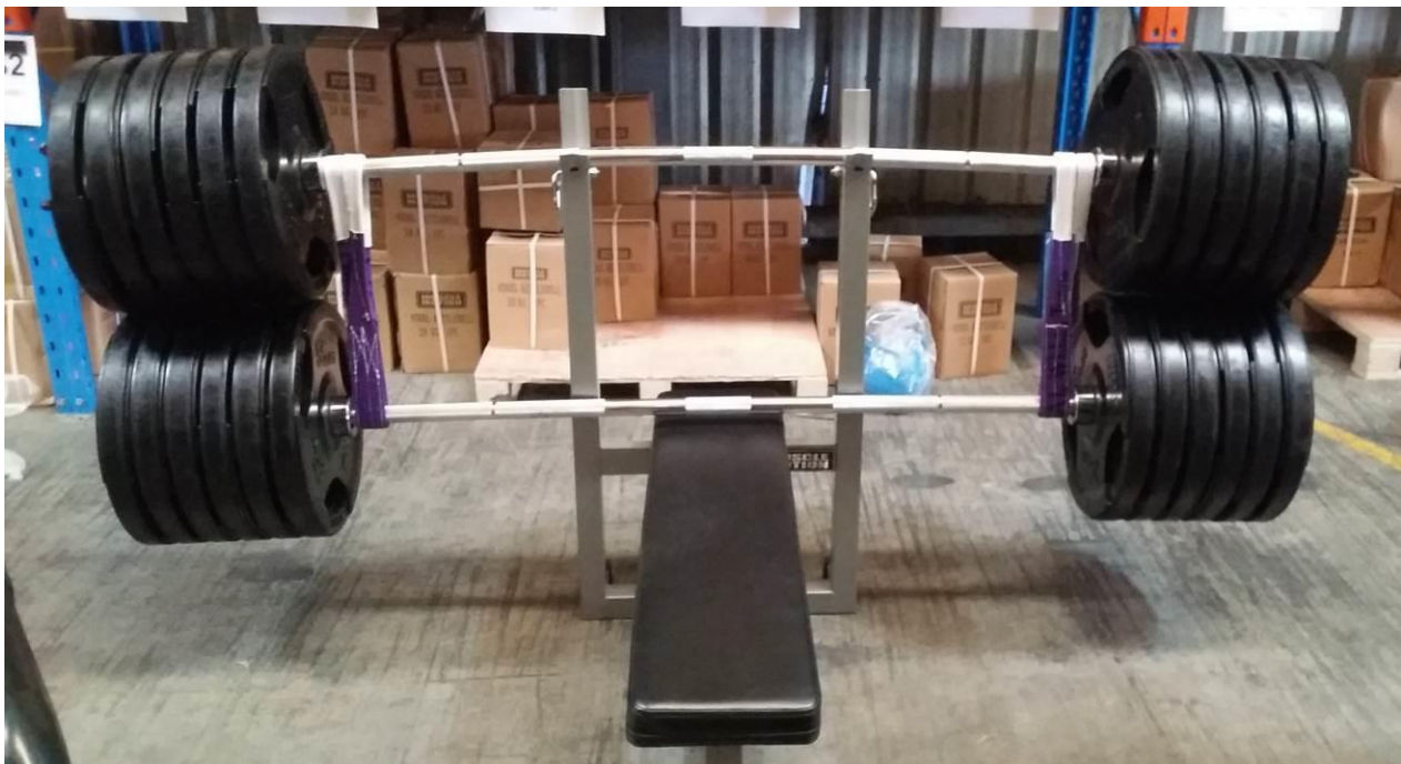
Figure: 3 Subject: View of the fixed barbell stands with the distributed test load (621.80kg) applied.
