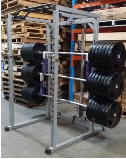
Figure: 2 Subject: View of the power rack with the distributed test load (1077.90kg) applied on the J hooks.
