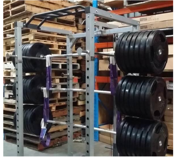
Figure: 3 Subject: View of the power rack with the distributed test load (1077.90kg) applied on the safety arms.
