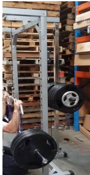
Figure: 5 Subject: View of the power rack with the distributed test load (203.60kg) applied on the high low pulley.
