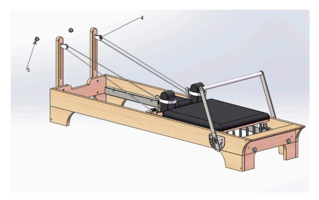
Step 5: Place 6- foot board and use 7- plum blossom nut to 8 - secure hole with bolt.
