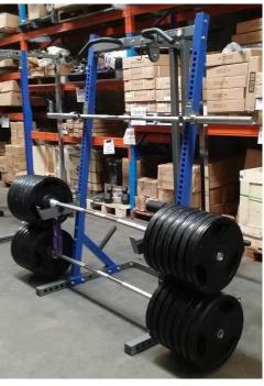
Figure: 2 Subject: View of the power rack with the distributed test load (71860kg) applied on the safety arms.
