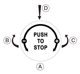
**Serial number A** is the brake knob, function ---- (+increase resistance -decrease resistance STOP stop movement)
