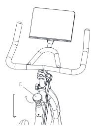
How to adjust the horizontal placement of bike.
