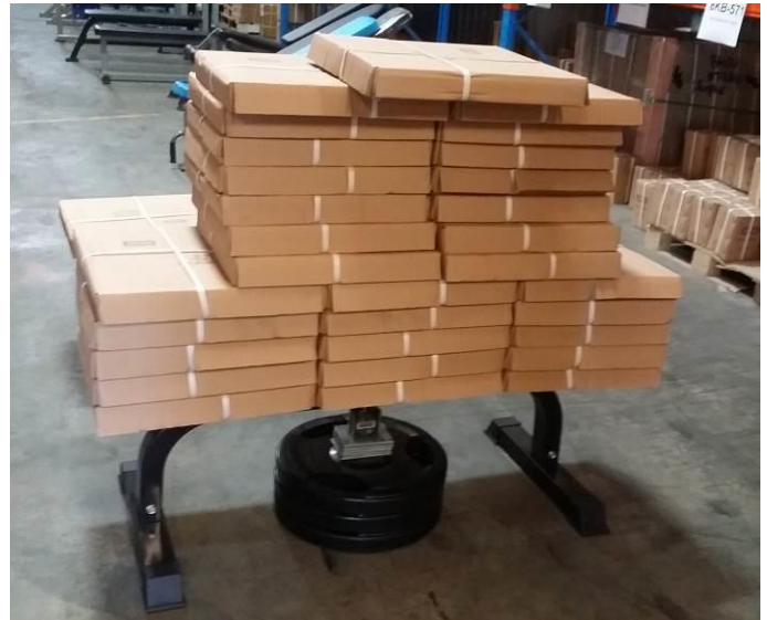
Figure: 2 Subject: View of the flat bench with the distributed test load applied.
