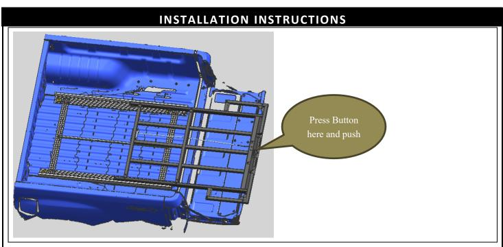
Step 5. Push the locking module from the rails on both sides of the slide tray base along to the hole position as bellow drawing and lock it with the hex bolt M8\_16;
