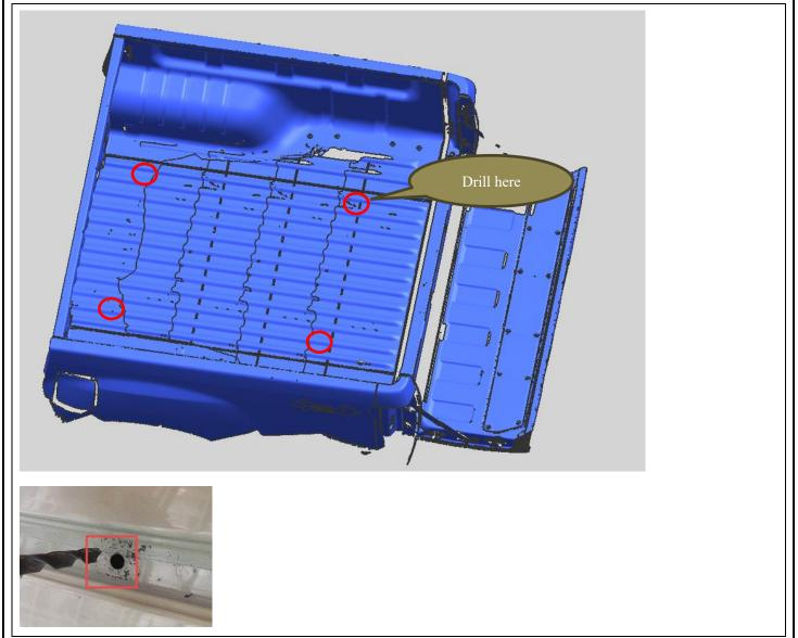
Step 2. Lock the base of slide tray by using 4 pcs of Hex Bolt M10\_65mm, 4 pcs of Spring Washer, 8 pcs of Extra-size Washer D12 and 4 pcs of Nuts M10;
