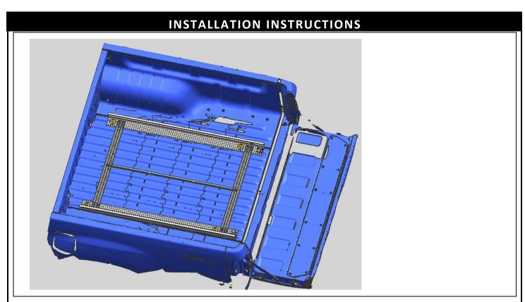
Step 3、Push the bearings on both sides of the Slide tray mounting bracket into the position halfway along the rail on both sides of the slide tray base; (Remark: Please keep pressing the button on the handle while pushing the mounting bracket of slide tray.)
