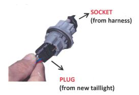
6. Twist all 3 sockets till they are securely connected to the new tail light housing. Please fix the 3 metal fixing plates by a screw dirver.
