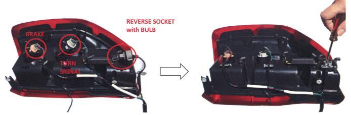
7. Align the mounting gaskets and set the new tail light onto the car. Fix the 2 screws (from step 1) firmly with the tail light.
