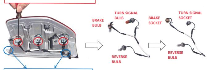
We also need to use the 2 taillight retainers from the OEM tail light, please remove them and install them onto the new tail light accordingly (as shown in below blue circles).
