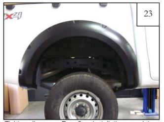
Tighten all screws. Rear flare installation complete.
