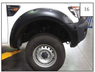
Tighten all screws. Front flare installation complete.
