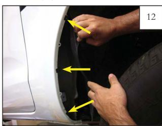
Peel back the rear wheel well liner and install three (3) supplied clips (CL1-0022) at the three locations indicated. Replace liner to original position.
