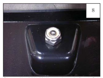
Place a Nut (NU1-0019) over the end of each Bolt and tighten, using a 1/2" wrench for the Nut and a T-45 Torx Bit for the Bolt. Repeat for remaining pockets.
