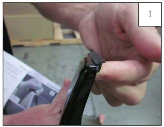
Peel two to three inches of red vinyl backing away from tpo gasket (GP1-0007) tape. Applying the adhesive side of the tpo gasket to the inner side of the flare, affix the tpo gasket to the top edge of the flare (the portion that comes in contact with the vehicle).
