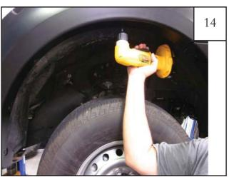
While using an electric drill install one (1) supplied self tapping screw (SW1-0066) into the center top location of flare and into sheet metal using hole in flare as a guide.
