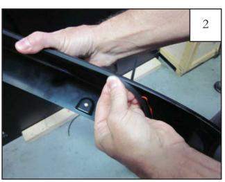
Press tpo gasket into place along the top edge of the flare in one-foot increments, pulling red vinyl backing free as you continue to work your way around the top edge of the flare.
