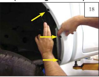
Peel back the front wheel well liner and install three (3) supplied clips (CL1-0022) at the three locations indicated. Replace liner to original position.
