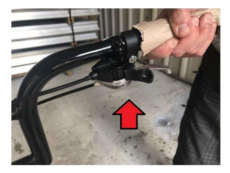
Here is how the shifter should look when turned to the correct position...
