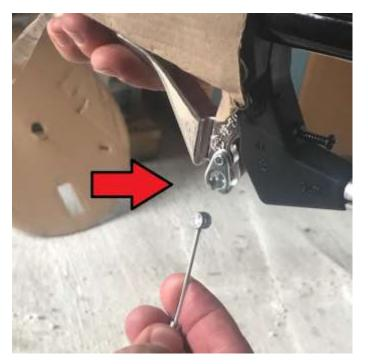
Step 2: Insert the cable into the connector as shown below:
