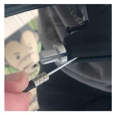
Step 4: Fully seat the cable into the lever and turn the nut to close the opening as show below:
