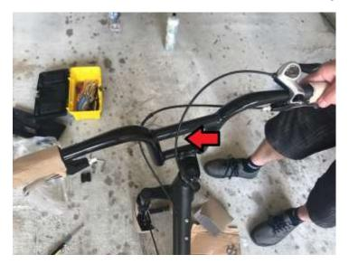
In order to get both cables in front of the bar, you may need to untangle the cables by slipping the handlebar through the cables as shown below...
