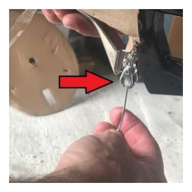
Step 3: Line-up the nut and barrel adjuster on the lever so that the open slot is exposed as shown here:
