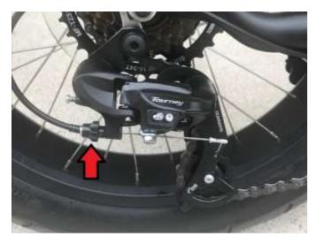
After adjusting take the bike for another test ride and see if you are able to shift into all 7 gears. If not, then the next step is to adjust the derailleur cable (#2 below). To do this, begin by loosening the bolt (#1 below) to provide a bit more slack in the cable. Now re-tighten the bolt.
