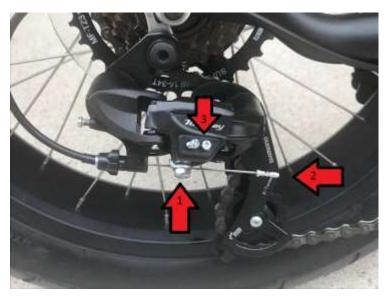
Take another test ride and shift through all 7 gears. It should now work. If not, repeat the process to make further adjustments to the cable tension. If the bike is shifting into all 7 gears but you hear a slight grinding sound in the chain, you can make subtle adjustments to the position of the derailleur by turning
