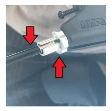
Step 5: Check to make sure both ends of the cable are fully seated (at the lever and at the brake caliper attached to the front wheel fork). Now engage/pull on the brake lever. Does the brake engage and stop the wheel about mid-pull? If so, stop here as the job is complete. If the brake lever instead goes all the way to the grip, then you'll need to perform an additional step.
