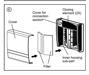
Mount the cover for the electrical connection section and insert the closing element on top!!
