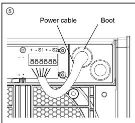
Connect the ventilation unit! (Connection plan, refer to p 5)
