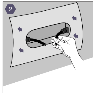
Cut the cable at an angle and pierce through the membrane of the integrated ELECTRISEAL BOX.
