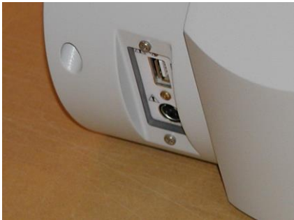
Figure 34 Location of the Printer output on the NucleoCounter
