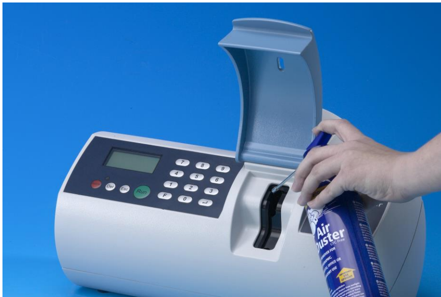
Figure 27. Removal of dust from the insertion slit using compressed air. Never use the container in a horizontal position and preferable do not use it at an angle greater than shown in the figure.
