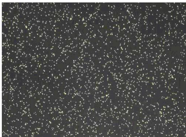
Figure 4. Fluorescent image (from NucleoView PC software) of cell DNA contained in the measurement chamber of a NucleoCassette
