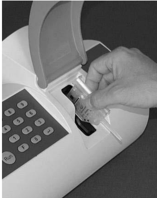
Figure 12. Illustration of how to grip and insert the cassette into the insertion slit
