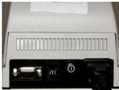
Figure 3 Location of the Serial connector on the PCNEOS printer (to the left).
