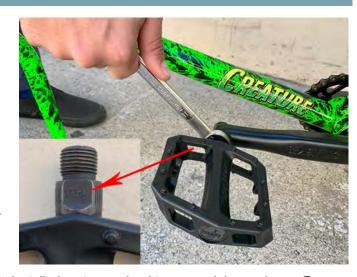
Note: You will damage the threads in the crank arms if you thread the wrong pedal into the wrong crank arm.
