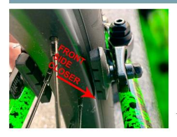
Adjust the front of the brake pads so they make contact with the rim first, there should be approximately 1mm gap on the other end. This will lessen the chance of rim squeal and improve your braking.
