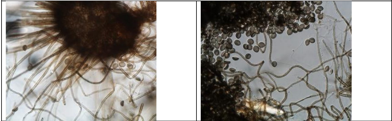
Chaetomium globosum Plywood Control Micrographs / Surface Sample
