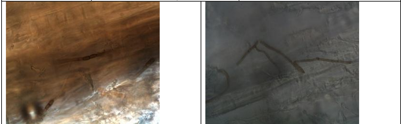
Ulocladium chartarum Plywood Bleach Treatment / Sub Surface Sample
