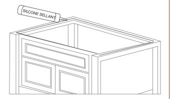
Inspect intallation area and make sure cabinet is secured properly. Apply silicone sealant around the topside of the cabinet's edge using a caulking gun.
