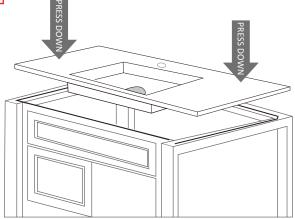
Connect the water supply to the faucet according to faucet instructions. Attach drain pipe assembly. Use clear or color matched silicone to seal drain.
