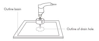
Cut or drill out the drain opening on the countertop using the appropriate drill by following the drain opening cut line as illustrated.
