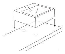
Measure outside perimeter of drain opening and mark countertop. Temporarily place the basin on the counter top to check for fit.
