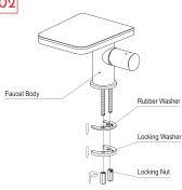
Remove locking nuts, locking washer and rubber washer from faucet body in turn.
