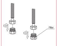
Remove the filter from the braided hose. Attention to the filter net in the filter.
