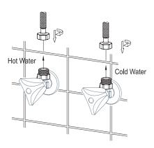
Connect the filter and braided hose. the red hose corresponds to hot water and blue hose corresponds to cold water. (Red on the left and blue on the right)
