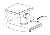
After the installation is complete, run water for inspection. The figure is for the case when the handle is turned on.
