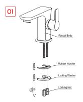
Remove the locking nut, locking washer and rubber washer from the faucet body.
