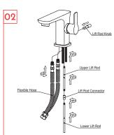
Connect the upper lift rod and lower lift rod. Put the lift rod knob into the slot in the back of faucet body to connect with the upper lift rod. Screw the flexible hoses (attention to the red and blue notes).
