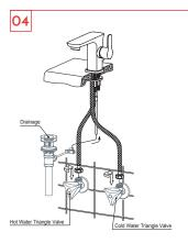
Connect the flexible hoses with triangle valves (red on the left and blue on the right). Connect the lift rod with drainage.
