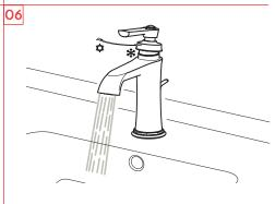
After installation, flow water to check if the installation is qualified. The figure displays open state of handle.
