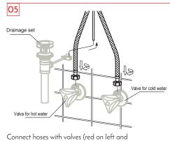
blue on right), connect lift rods with drainage set.
