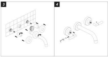
3.As the picture shows. First set the spout into the decoration Then wrap the raw material tape and screw it into the embedded body Finally screw in the two spool position sheath and decorative cover
