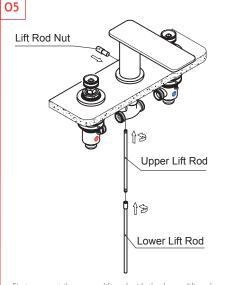
First connect the upper lift rod with the lower lift rod. Then insert the lift rod nut into the slot at the back of the faucet body to connect with the upper lift rod.
