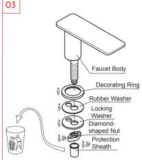
Take off the following from the faucet body accordingly: the protection sheath, diamond-shaped nut,locking washer, rubber washer and deco rings.
