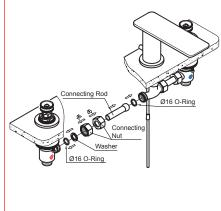
Use the connecting rod to connect the two inlet valve bodies and the three-way inlet. Tighten them with connecting nuts.
