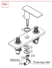
Put the decorating ring onto the faucet body and then place the faucet body downward through the basin deck. Then put on the rubber washer and locking washer, tightened by diamond-shaped nut and setscrew. Connect the three-way inlet.
