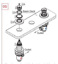
Place the two inlet valve bodies (red on the left and blue on the right) upward through the basin deck with the outlet holes facing against each other. Tighten on the decorating rings. Put on the plastic spacer (red for the left and blue for the right) and then tighten the hex nuts. Install back the handle core and
