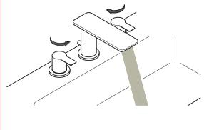
After installation, turn on water to check if everything is complete. Attention to cold water on the right and hot water on the left. The diagram shows water flow when the handles are turned on.
