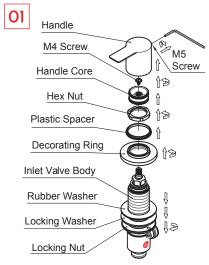
Loosen the M5 screw first. Take off from the inlet valve bodies the following one by one: handle, M4 screw, handle core, hex hut, plastic spacer and decorating ring. Screw off the locking nuts to the bottom.
