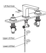
Connect the upper lift rod and lower lift rod. Put the lift rod knob into the slot in the back of faucet body to connect with the upper lift rod.
