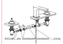
Connect two inlet valves and tee pipe coupling with connecting rod. Tighten the connecting nuts.
