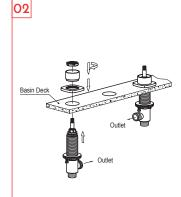
Unscrew the M5 screw. Remove the handle, screw, handle core, plastic space ring, clamp ring, handle escutcheon and sub-escutcheon from two inlet valves. And screw the locking nut to the bottom.
