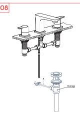
Connect the lift rod and drainage.
