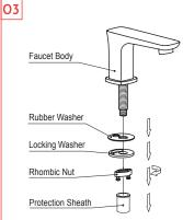
Remove the protection sheath, rhombic nut, locking washer and rubber washer from the faucet body.
