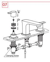
Tighten the locking nut and clamping screws in order. Then reinstall the plastic space ring, handle core, screw and handwheel in turn and fix with M5 screw. (Make sure that the handle printed sun mark is installed on the left and the handle with snow mark is installed on the right.)
