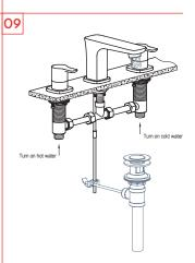
After installation, flow water for inspection. The figure is for the case when the handle is turned on.
