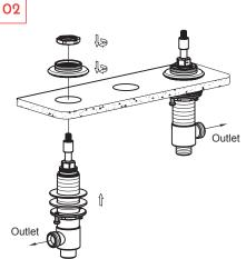
Pass two inlet valves (red on left and blue on right) from down upwards through holes of basin, keep outlets of inlet valves toward the opposite, install and tighten base, then fix hexagonal nut.
