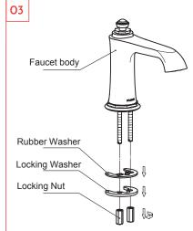
Remove locking nut, locking washer and rubber washer from faucet body.
