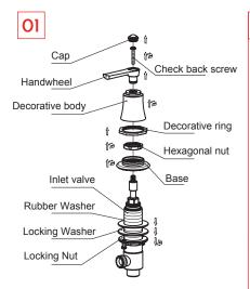
Pick out cap by a sharp point tool, remove check back screws, handwheels, decorative bodies, decorativerings, hexagonal nuts and bases from two inlet valves in turn, screw locking nuts to the hottom
