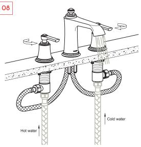
After installation, flow water (hot on left and cold on right) to check if the installation is qualified. The figure displays open state of handwheels.
