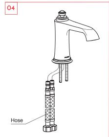
Connect hoses (Torque  $\leq 5N \cdot m$ ) as red(hot) on left and blue(cold) on right.
