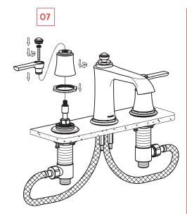
Pad decorative rings and tighten decorative body. Install handwheels (Note:red on left and blue on right), fix with check backscrews and insert cap.
