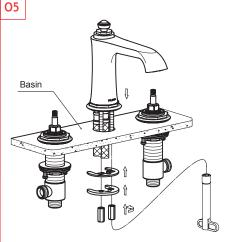
Pass faucet body from up downwards through hole of basin, pad rubber washer and locking washer, fix with locking nuts.
