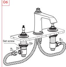
Connect hoses to inlet valves, tighten locking nuts and set screws on inlet valves in turn.
