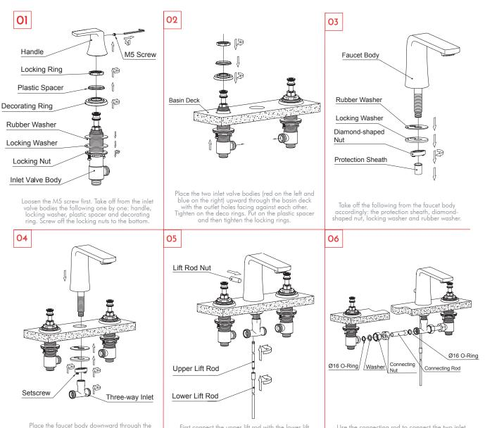
Place the faucet body downward through the basin deck. Then put on the rubber washer and locking washer, tightened by diamond-shaped nut and setscrew. Connect the three-way inlet.
