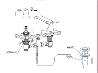
Loosen the M5 screw first. Take off from the inlet valve bodies the following one by one: handle, locking washer, plastic spacer and decorating ring. Screw off the locking nuts to the bottom.
