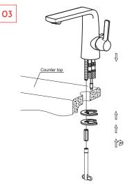
Pass the mixer body through the counter top, install the rubber washer and the mounting washer. Tighten them with the locking nut.
