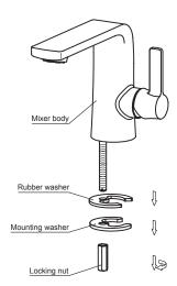
Disassemble the locking nut, mounting washer and rubber washer from the mixer body in turn.
