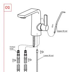
Insert the upper lift rod into the slot on the back of the mixer body. Connect the upper lift rod with the lower lift lod. Screw the knitted hose withred(hot) in front and bule(cold) in back.
