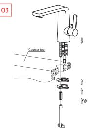
Pass the mixer body through the counter top, install the rubber washer and the mounting washer. Tighten them with the locking nut.
