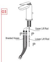
Put the upper lift rod into the slot on the back of faucet body to connect with the lower lift rod. Screw the braided hoses. Attention to the red on the left and the blue on the right.
