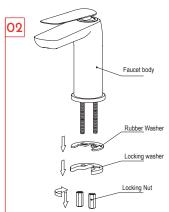
Remove the locking nut, locking washer and rubber washer from the faucet body.
