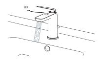
After installation, run water for inspection. The figure is for the case when the handle is turned on.
