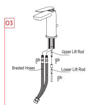
Put the upper lift rod into the slot on the back of faucet body to connect with the lower lift rod. Screw the braided hoses.
