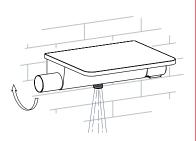
Turn handwheel convexity to the back, water runs from shower connection.
