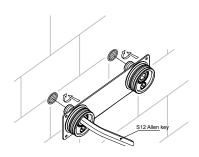
Place two offset connectors through locating plate and screw them into pipe joint, slightly tighten inlet thread joint by \$12 allen key.
