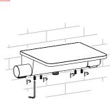
Make sure faucet body close to the wall, then tighten M6 screws.
