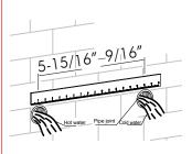
Lay hot and cold water pipes in the wall about 600mm above the floor, with hot on left and cold on right and 150mm distance between them.Run water to get rid of dirt in pipes.
