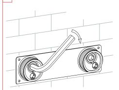
Tighten inlet thread joint with \$12 allen key.
