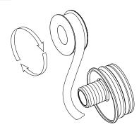
art off Wrap two offset connectors with teflon tape.
