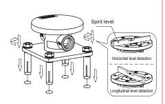
Insert expansion bolts into holes on the floor (Note:cold water inlet which printed with "COLD" mark on inlet base faces to the bath-tub), adjust the top surface of inlet base to level position with spirit level and tighten with hexnut.
