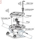
Connect inlet base with cold and hot water inlet pipe,cold water inlet faces to bathtub, hot water inlet back against bathtub(means front cold and back hot),wrap connectors with teflon tape.Note to flow water to get rid of dirt in pipes.Remove protection sheath,insert plug into outlet of inlet base and fix with flange.
