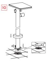
Take off protection sheath, insert inner pipe vertically into outlet of inlet base, connect flange and inlet base with locking screw, tighten with allen key. Close escutcheon to the floor.
