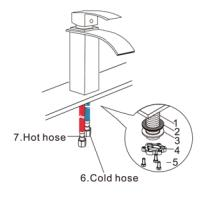
2. Screw rubber washer(2), metal washer(3) and lock nut(4) onto the pipe(1).
