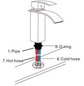
1.Remove the Rubber washer (2), Metal (3) and lock nut (4) from the faucet.
