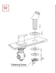
Place shower holder through the escutcheon and bathtub deck hole. Reinstall parts together again and tighten the locking nut with fastening screw.
