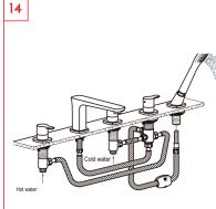
After installation, flow water for inspection. The figure is for the case when the handle is turned on.
