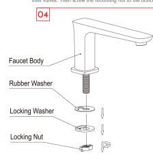
Remove the locking nut, locking washer and rubber washer from the faucet body.
