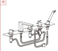
Turn the diverter handwheel to the left for bath pout water.
