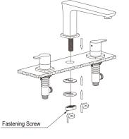
Place the faucet body through the bathtub deck hole. Install the rubber washer and locking washer. Screw the locking nut and tighten it with fastening screw.
