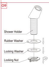
Remove the locking nut, locking washer and rubber washer from the shower holder.
