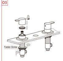
Screw the mounting nut and fasten screw tightly. Then put on plastic spacing. Install handwheel (attention: the hanswheel wich "sun" mark is printed is installed on the left and handwheel wich "snow" mark is printed is installed on the right) and fix it with M5 screw.
