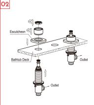
Place two inlet valves (red on the left and blue on the right) through the bathtub deck and keep two outlet towards each other. Put on the decorative body and screw the escutcheon. Tighten them with mounting nuts.
