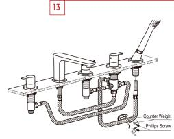
Put the counter wight on the flexible hose in plastic material at the proper position. (Make sure the hose can easily be pulled out).
