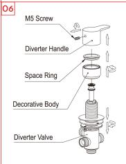
Remove the diverter handle, space ring and handle escutcheon from the diverter valve in turn. Screw the locking nut to the bottom.
