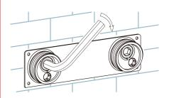
Adjust the S-connector sets parallel with the locating plate with S12 wrench. Check it by level ruler and screw up the screw joints (Fig.7, Fig.8 and Fig.9).
