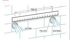
Install the cold and hot water pipes in the wall at the height of 600mm. The distance between is 150mm with the hot water on the left and the cold water on the right
