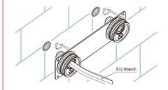
Wrap the two S-connectors with Teflon tape and put them through the locating plate and screw them into the pipe joint. Tighten them with S12 wrench (Fig.5 and Fig.6)
