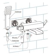
Put on the faucet body to the S-connectors against the wall, tightened them with 4 M4 screws. Connect the handshower and the faucet body with the flexible hose. the installation is finished.
