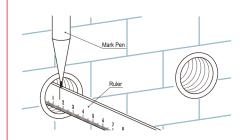
Measure the depth of thread joint with ruler and make marks on the wall with marked pen based on the wall
