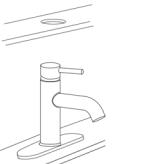
2. Screw rubber washer(2), metal washer(3) and lock nut(4) onto the pipe(1). And then connect water supply(not included) on the hot hose(7) and cold hose(6).
