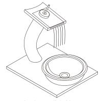
3) Open the hot and cold water supplies. Check for leaks. Turn on faucet handle for one minute to flush debris from faucet.
