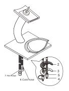
2) Tighten lock nut (5), metal washer (3) and rubber washer (2). And then connect water supply (not included) on the hot hose (7) and cold hose (6).
