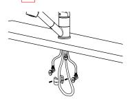
Attach Weights to the pull-out hose using screws at the proper point of the hose. Be noted Weights are optional.
