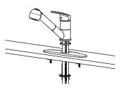
Make sure the O-RING is placed onto the bottom of Base Ring. Install faucet through Deck Plate. From underside sink, put Plastic Washer and Mounting Nut. Position faucet on sink properly and tighten Mounting Nut. 03
