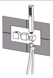
Connect the shower hosewith hand shower and hose connector to complete the installation.
