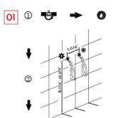
Flush the water supply lines throughly to drain debris and impurities. Shut off the water before installation. 02
